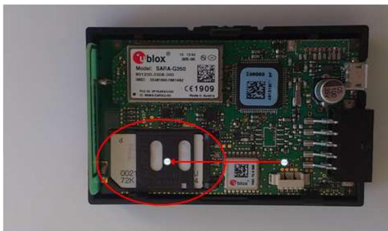
Figure 4: Where to insert the SIM Card
