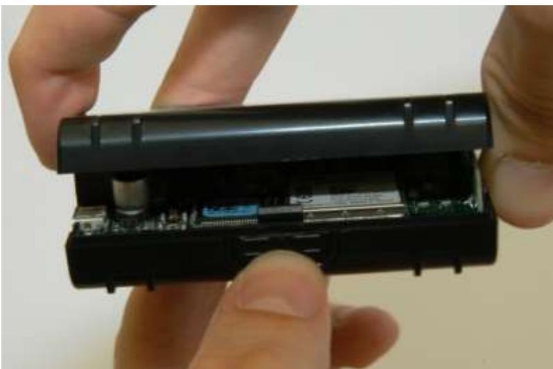
Figure 2: How to open the SBC-AVL Housing
