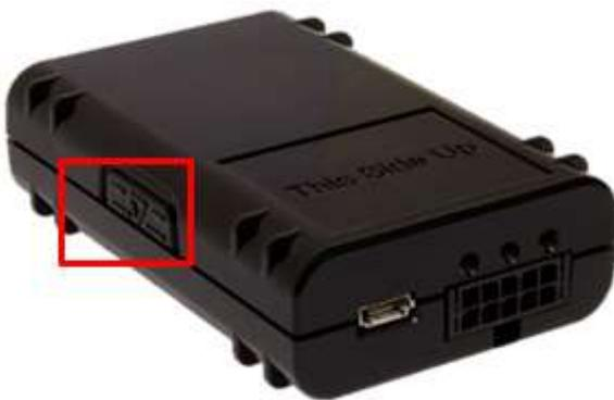
Figure 1: The button to open the SBC-AVL Housing
