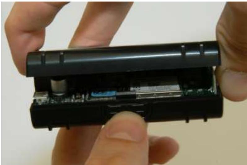
Figure 5: How to close the SBC- AVL Housing
